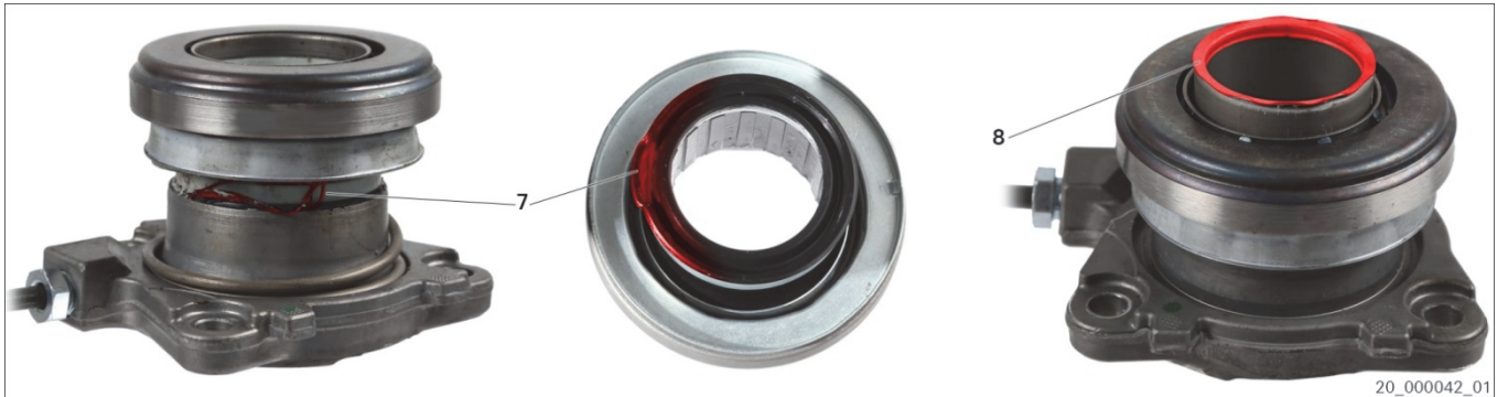
Fig. 2: Lipped seal ring is sheared
