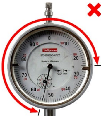
Fig. 3: Lateral run-out \geq 0.5 mm
