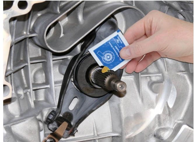
Fig. 2: Lightly grease the splines of the transmission input shaft
