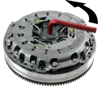
Fig. 3: Unscrew locking piece
